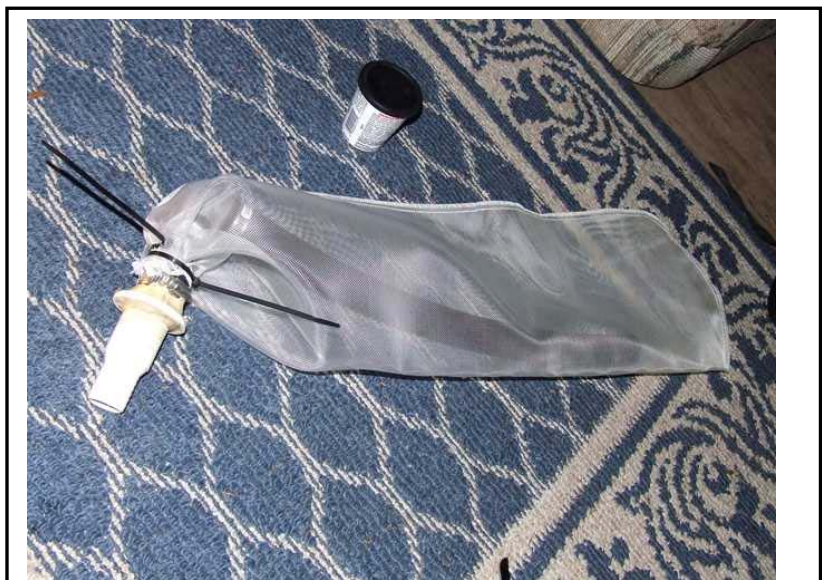
The outlet system to be installed in the olive barrel (through-hull fitting attached to a pipe with holes drilled into it and covered with a filter bag)
